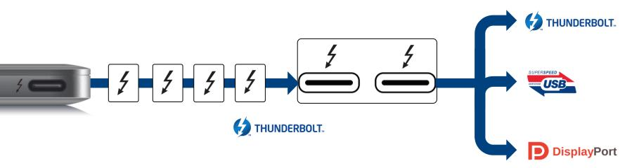
Second device port operates the same as computer port and supports Thunderbolt, USB, and DisplayPort devices
