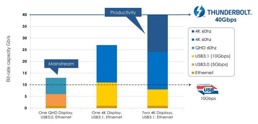
Showing max bandwidth for each protocol listed - many other protocols are possible depending on dock configuration (eSATA, card slots, Firewire, HDMI, Wi-Gig)
